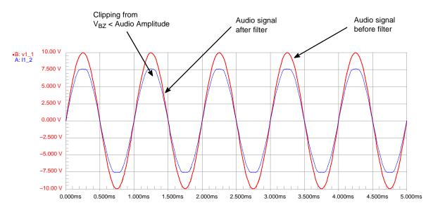
Figure 16. Vz < Audio amplitude with no DC offset. If the  $V_{WRM}$  is significantly less than the peak voltage of the audio signal, the signal will be clipped at  $V_{BZ} + V_{F}$ . In this example the amplitude of the audio voltage is 10 V, while  $V_{BZ} + V_{F}$  of the filter is about than 7.5 V. The breakdown voltage of the ESD/EMI Filter should be closer to 14 V for both directions.
