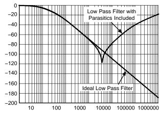
Figure 19. Ideal vs. Real at 50  $\Omega$ . Because of the parasitics in the surface mount components, the insertion loss characteristics of the filter make the filter behave like a band rejection filter and not a low pass filter. Frequency in kHz.
