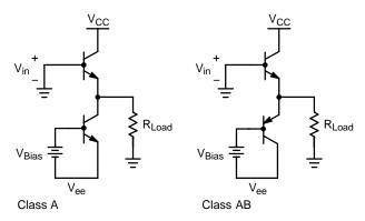
Figure 3. Basic configurations of a Class A and Class AB output stages. The class A is one of the more simple configurations, but is very inefficient. The Class AB has similar efficiencies to the Class B, but is compensated such that there is no crossover distortion.
