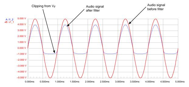
Figure 12. Vz < Audio amplitude with no DC offset. If unidirectional TVS diodes are used on audio lines that are not DC offset, such that the audio signal may cause the TVS diodes to become forward bias and clip the audio signal below the V<sub>F</sub> of the diode.
