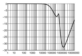
Figure 21. EMI filter at 50  $\Omega$ . The purpose of the EMI filter is to filter out signals in the range of 800 MHz to 2.5 GHz. Frequency in kHz.
