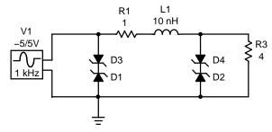
Figure 13. Basic Configuration of an ESD/EMI Filter using Bidirectional TVS Diodes
