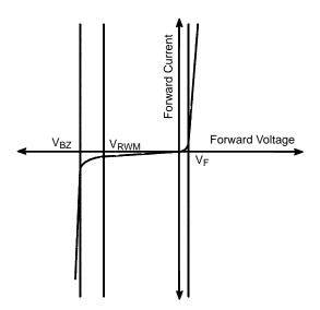
Figure 9. The IV characteristics of a TVS diode are typical for Zener diodes. The areas to note typically are the  $V_{BZ}$  and  $V_{RWM}$ .
