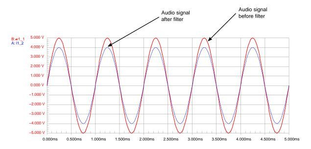
Figure 15. Vz > Audio amplitude with no DC offset. In this example the audio signal has amplitude of 5.0 V with no DC offset. The only attenuation to the signal should be caused by the series resistance of the filter. In this case the peak audio amplitude is less than the  $V_{WRM}$ .
