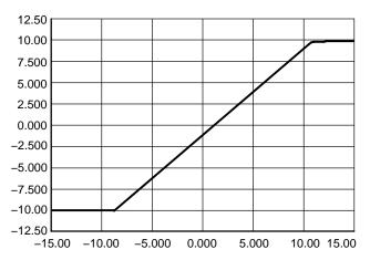
Figure 4. Basic Transfer Characteristic of either a Class A or Class AB Audio Output Stage
