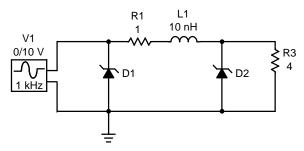
Figure 8. Basic Configuration of an ESD/EMI Filter using Unidirectional TVS Diodes
