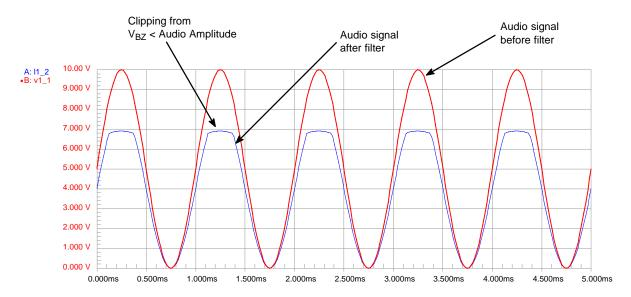
Figure 11.  $V_{WRM}$  < Audio amplitude with DC offset. If the  $V_{WRM}$  is significantly less than the peak voltage of the audio signal, the signal will be clipped at  $V_{BZ}$ . In this example where the peak audio voltage is 10 V, while the  $V_{BZ}$  of the filter is less than 7.0 V. The breakdown voltage of the ESD/EMI Filter should be closer to 14 V.
