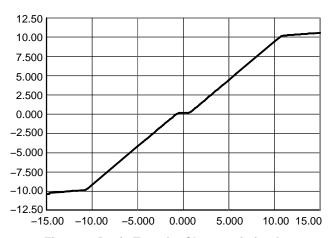
Figure 6. Basic Transfer Characteristic of a Class B Output Stage
