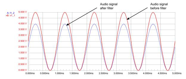
Figure 10.  $V_{WRM}$  > Audio amplitude with DC offset. In this example the audio signal has an amplitude of 2.5 V with a DC offset of 2.5 V. The only attenuation to the signal should be caused by the series resistance of the filter. In this case the peak audio amplitude is taken to the  $V_{WRM}$ . Ideally, the audio signal operates above the  $V_F$  of the TVS and below the  $V_{WRM}$ .
